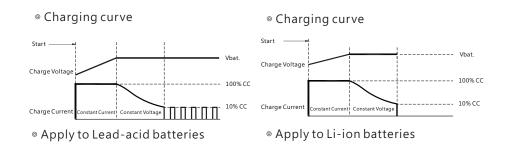
NOTE: In security applications, lead-acid batteries are generally used for floating charging. It is recommended that the charging voltage of the LAD should not exceed the floating charging voltage of the battery to ensure that the battery does not under long-term use.
