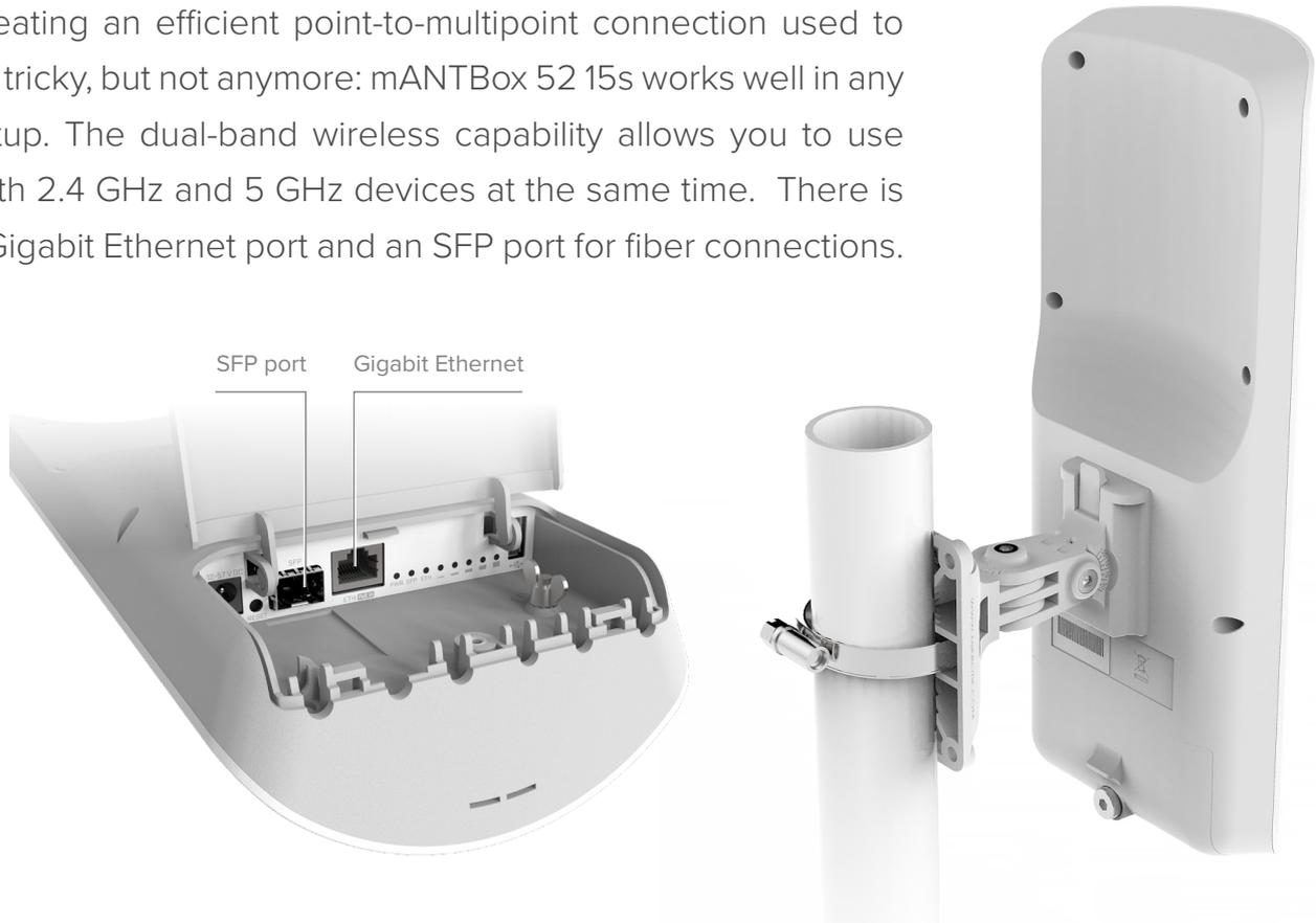
With mANTBox 52 15s you don't have to worry about power options – it supports 802.3af/at PoE-in. There is a Gigabit PoE injector and a standard DC power adapter included.
