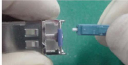
3. Cover unused optical connectors with protective caps, as shown in [Figure 14-5](#), and then lay out fibers on the fiber rack or coil them in a fiber management tray to prevent fibers from being squeezed.
