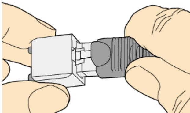
**Step 3** When you hear a click, the cable connector is completely inserted in the port. (The clip on the cable connector pops up to fix the connector in the port.) Pull the connector slightly and ensure that it is securely connected, as shown in [Figure 10-52](#).
