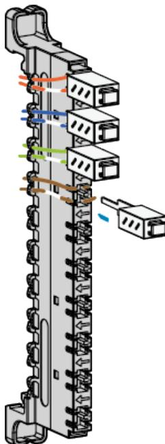
6. Install the cable management strip onto the cable management strip holder, making the end with a shorter hook face up and the end with longer hook face down, as shown in [Figure 6-11](#). Gently shake the cable management strip. If the cable management strip is still fixed on the holder, it is installed properly.
