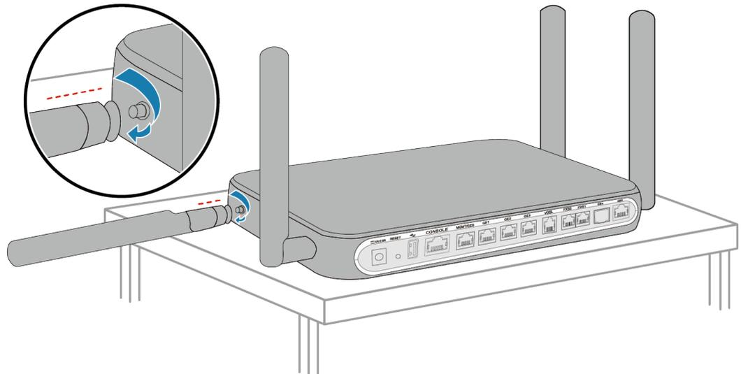
**Step 2** Adjust positions of the antennas to obtain the optimal wireless transmission and receiving performance. If the router is placed on a desk, make the primary antenna vertical to the desk and secondary antenna parallel to the desk.
