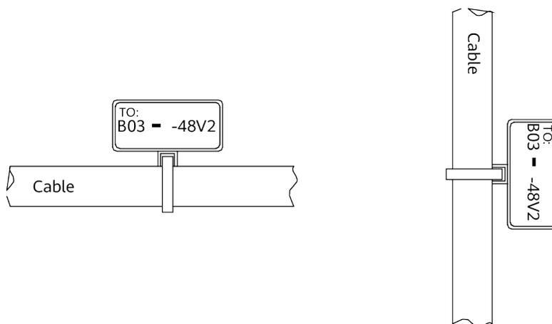
The identification card is on the top of the cable in horizontal cabling.
