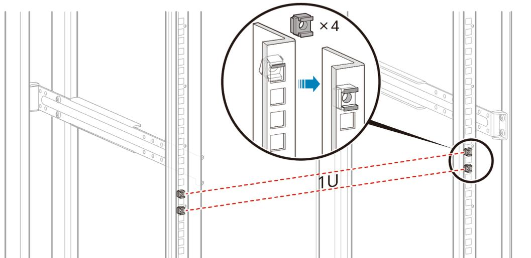
**Step 3** Move the router into the cabinet. Support the bottom of the router with one hand and tighten the M6 screws on the mounting brackets with the other hand. Tighten the lower screws first, and then the upper screws.
