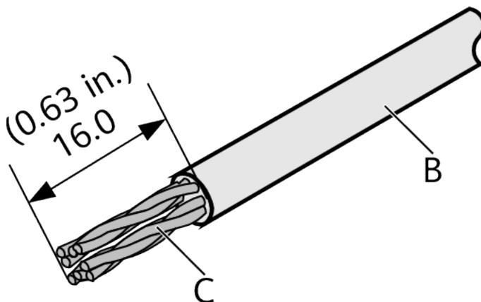
**Step 2** Align the four pairs of wires and cut the ends neatly, as shown in [Figure 10-30](#). The connections between the wires and the pins are listed in [Table 10-6](#).
