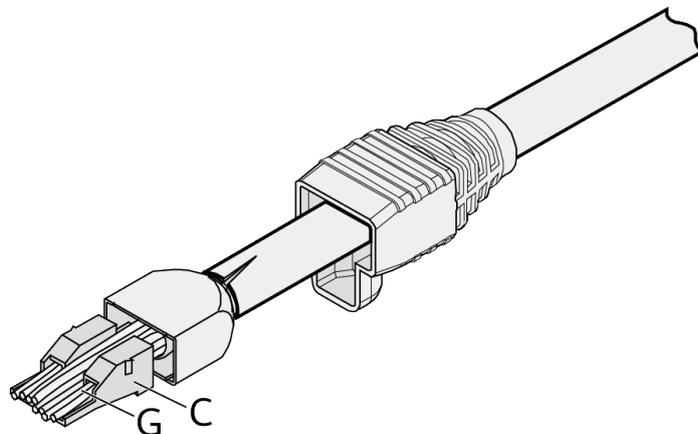
**Figure 10-23** Connections between wires and pins
