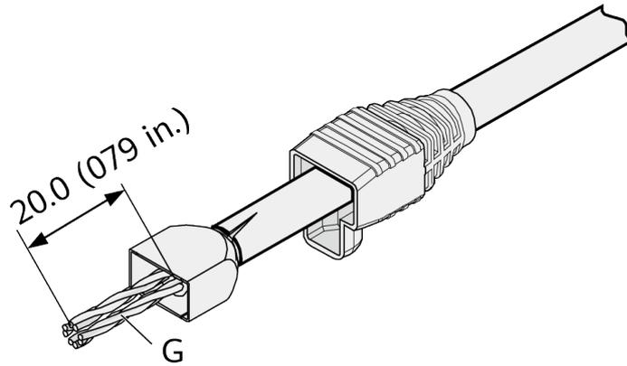
**Step 5** Lead the four pairs of twisted-pair wires through the wire holder, as shown in [Figure 10-20](#) and [Figure 10-21](#). Ensure that the colored wires are in the correct location in the cable.
