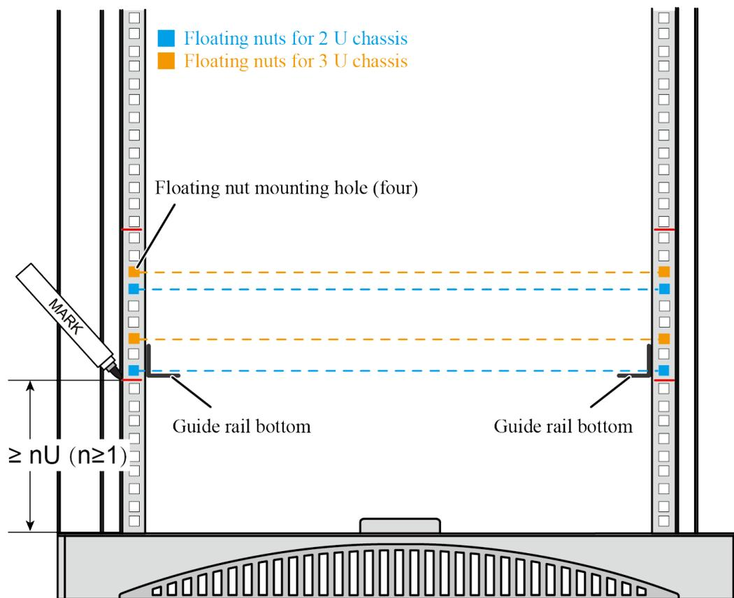
**Step 3** Install the floating nuts and L-shaped guide rails.
