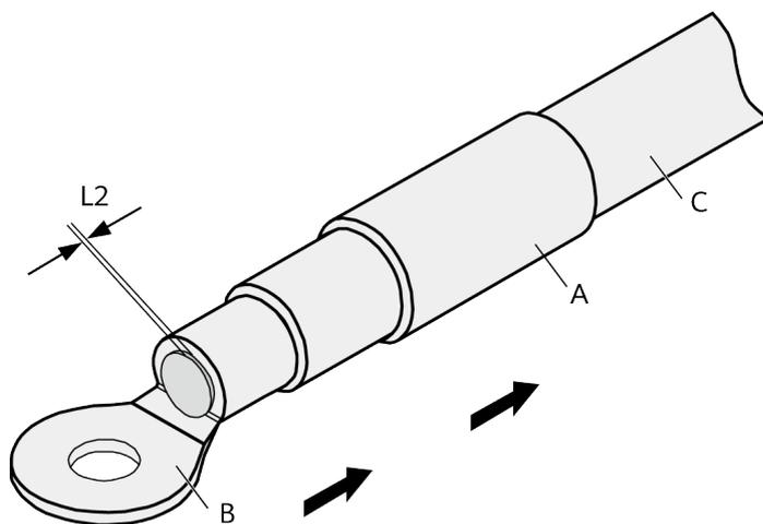
**Step 3** Put the OT terminal B onto the exposed conductor, and ensure that the OT terminal is in good contact with the insulation coating C, as shown in [Figure 10-3](#).
