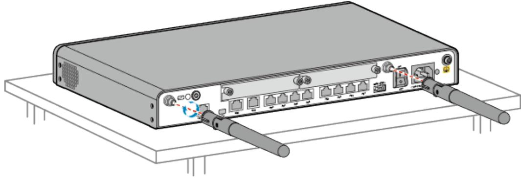
**Step 2** Adjust positions of the antennas to obtain the optimal wireless transmission and receiving performance.
