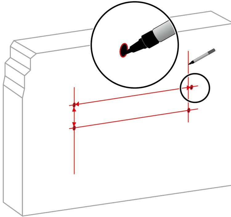
**Step 3** Drill holes and install mounting expansion bolts in the wall.
