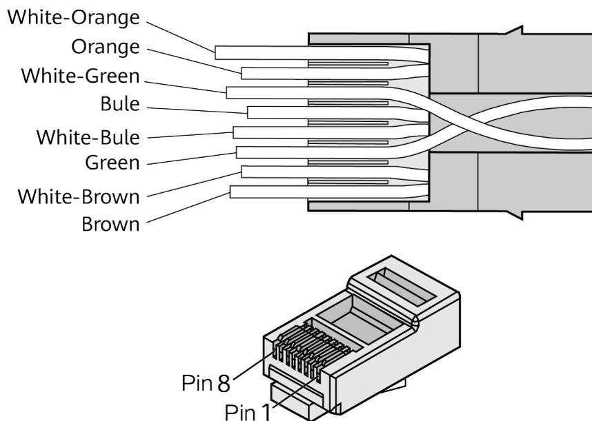
**Table 10-5** Connections between wires and pins (using a straight-through cable as an example)
