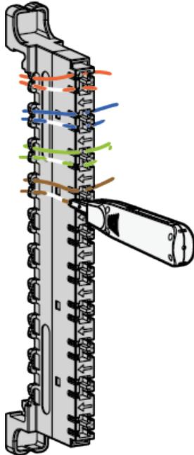
5. Install a protective unit on each wire slot with wires connected. Keep a protective unit vertical with a wire slot (with the diode of the protective unit facing the arrowhead on the wire slot), and insert the protective unit until it is completely in the wire slot, as shown in [Figure 7-11](#).
