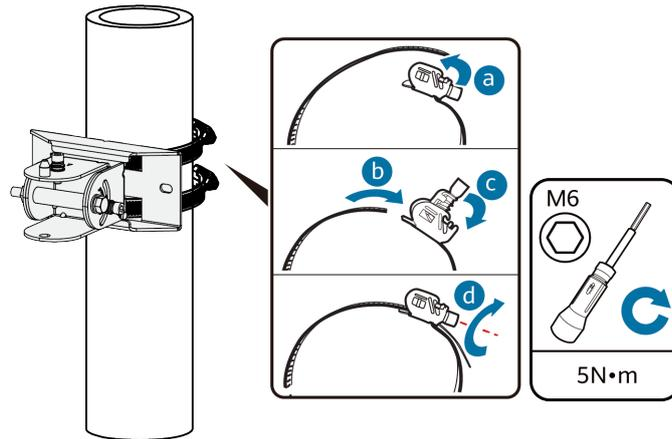
1. Use the M6 hex torque screwdriver to loosen screws on the hose clamp and lift the lid.
