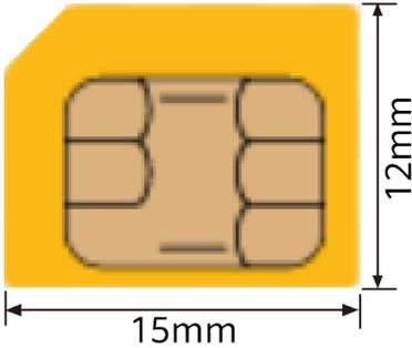
A yellow micro SIM card with a gold-colored chip. The dimensions are 15mm in width and 12mm in height.     |
