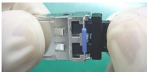
If no protective cap is available, use fibers to protect the optical module, as shown in [Figure 14-4](#).
