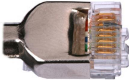
**Step 4** Check whether the contact strips and the plastic separators are well aligned and intact. If a separator is skewed and cannot be fixed, replace it with a new RJ45 connector. [Figure 10-36](#) shows an unqualified piece.
