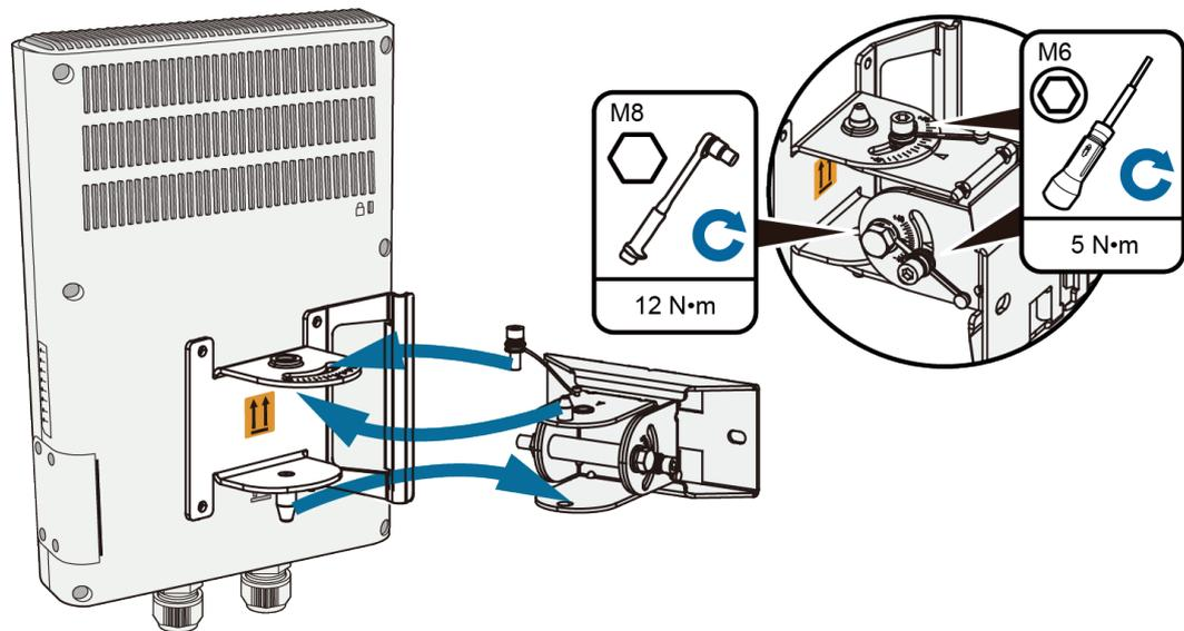
**Step 4** Loosen the two screws in the horizontal direction, adjust the horizontal and vertical angles of the device using the scale plate, and tighten all screws.
