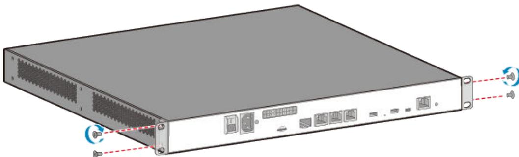
**Figure 6-2** Install rear mounting brackets
