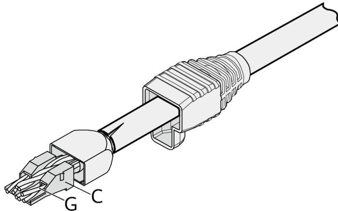
**Figure 10-21** Cable locations in a wire holder
