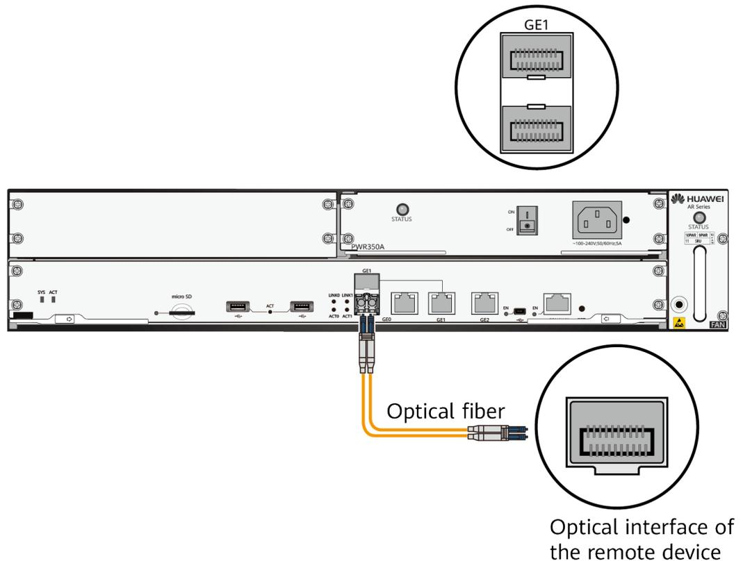
**Step 5** Arrange the optical fibers to make them parallel and bundle them with fiber binding tape at an interval of 150 mm to 300 mm.
