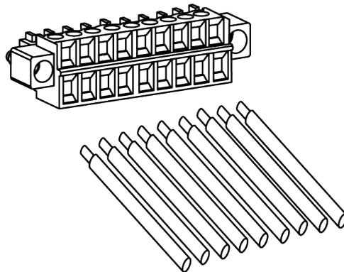
3. Tighten the screw on the wire hole with a flat-head screwdriver to lock the wire.
