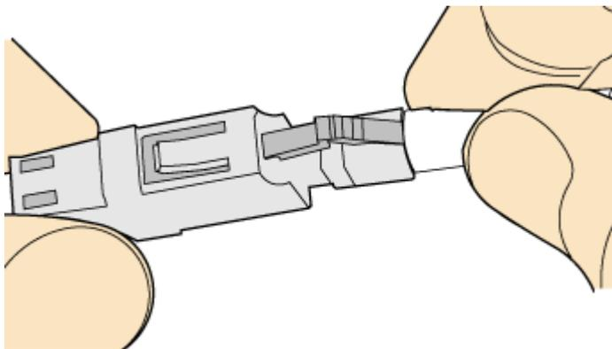
**Step 4** A clicking sound indicates that the male connector is locked, as shown in [Figure 10-64](#).
