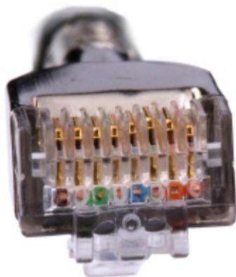
**Figure 10-33** Contact strips of the same height
