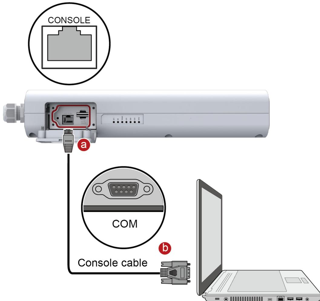
**Step 3** Start the terminal simulation software, create a connection, configure the connected port, and set communication parameters as follows.
