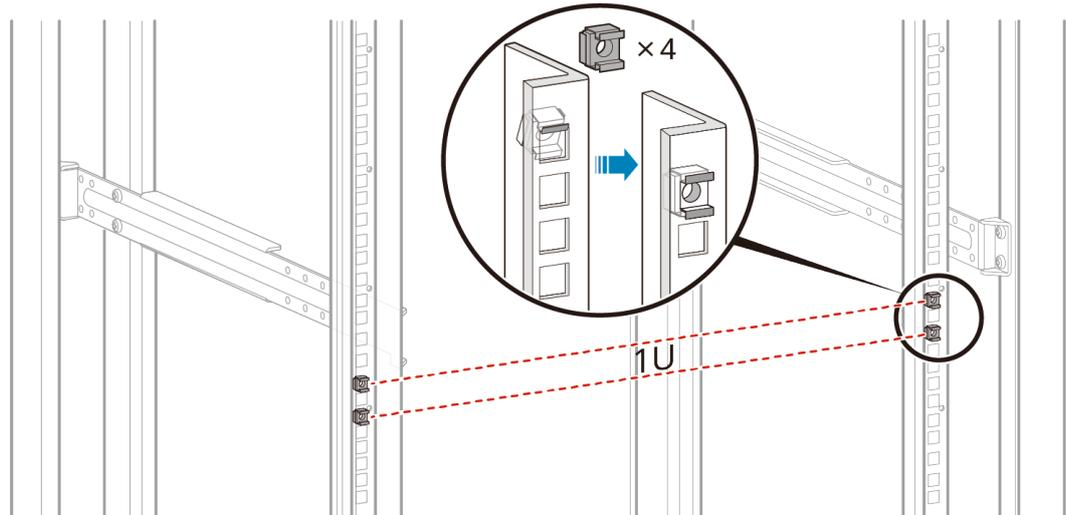
**Step 3** Move the router into the cabinet. Support the bottom of the router and tighten the M6 screws on the mounting brackets. Tighten the lower M6 screws first, and then the upper M6 screws.
