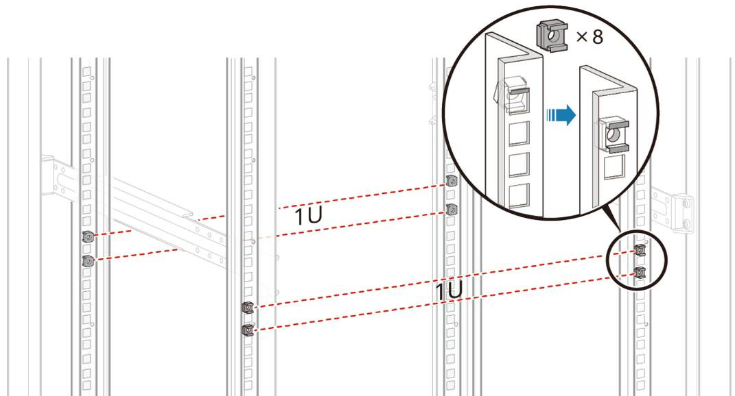
**Step 3** Fix the mounting bracket guide rails on the rear mounting rails.
