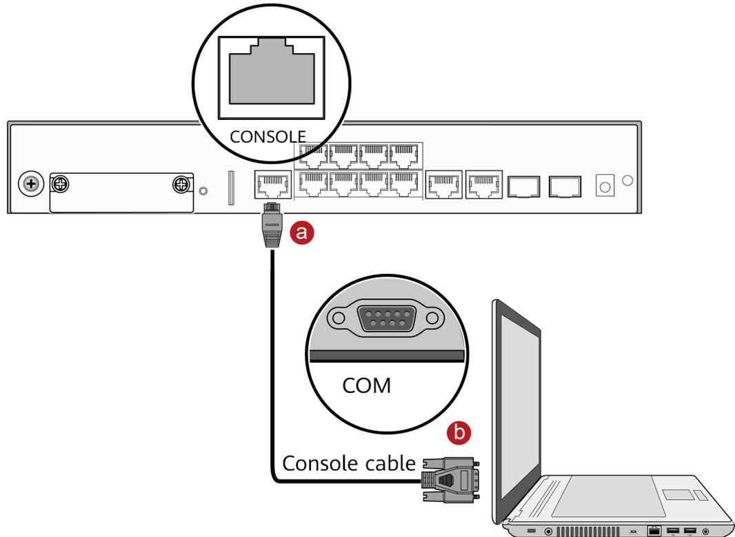
**Step 3** Start the terminal simulation software, create a connection, configure the connected port, and set communication parameters as follows.
