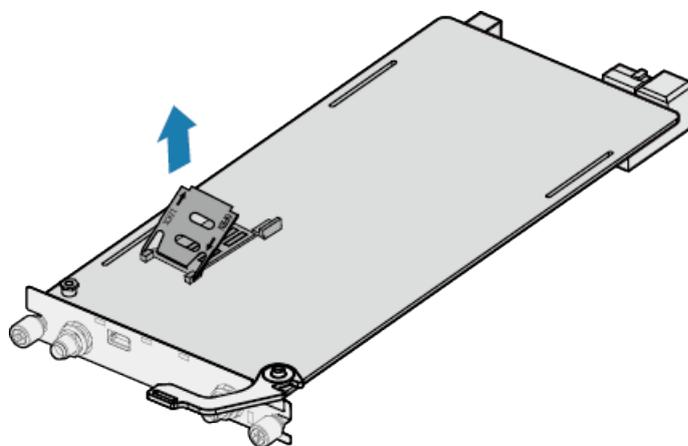
**Step 4** Insert a SIM card into the SIM card holder.
