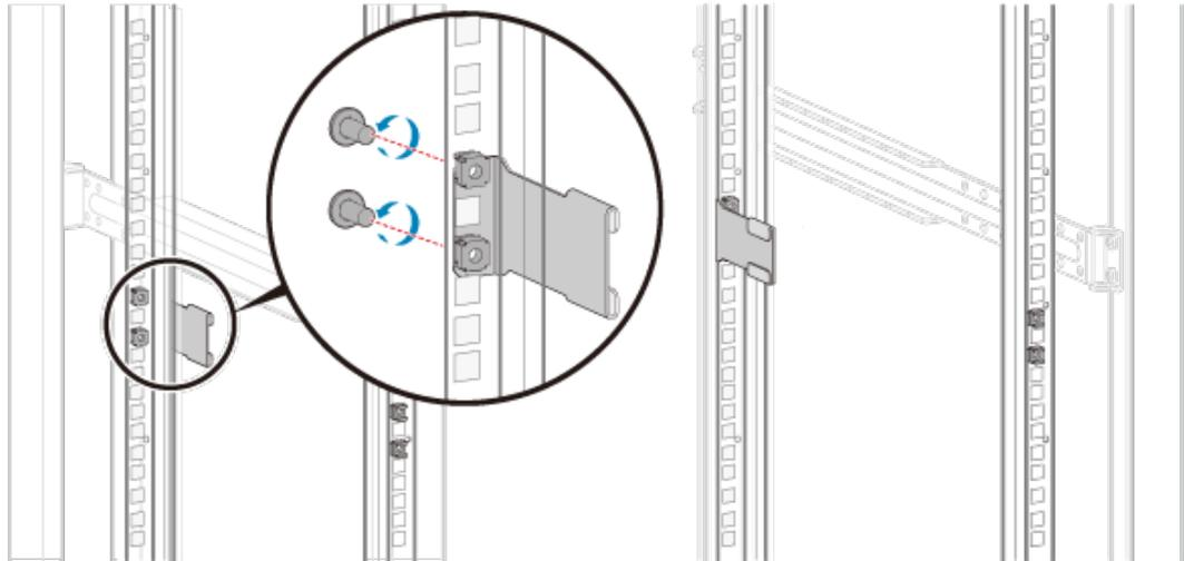
**Step 4** Install the router into the cabinet.
