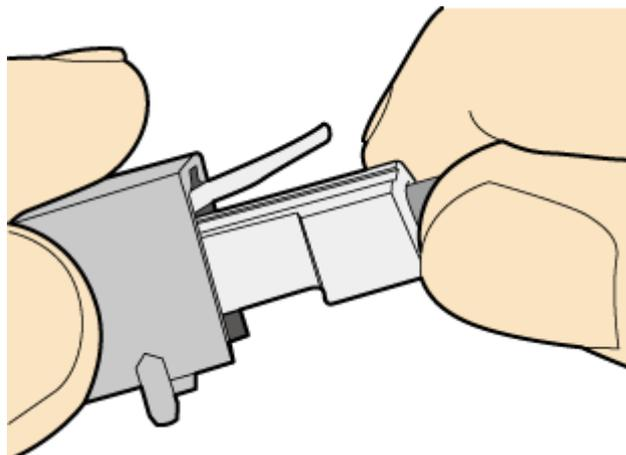
**Step 3** A crisp click indicates that the connector is locked by the locking key. Pull the connector slightly and ensure that it is securely connected. [Figure 10-56](#) shows an installed Ethernet connector.
