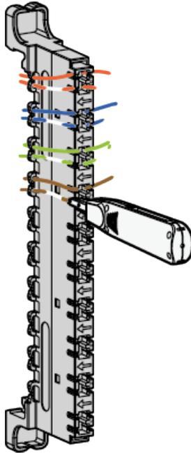
5. Install a protective unit on each wire slot with wires connected. Keep a protective unit vertical with a wire slot (with the diode of the protective unit facing the arrowhead on the wire slot), and insert the protective unit until it is completely in the wire slot, as shown in [Figure 6-10](#).
