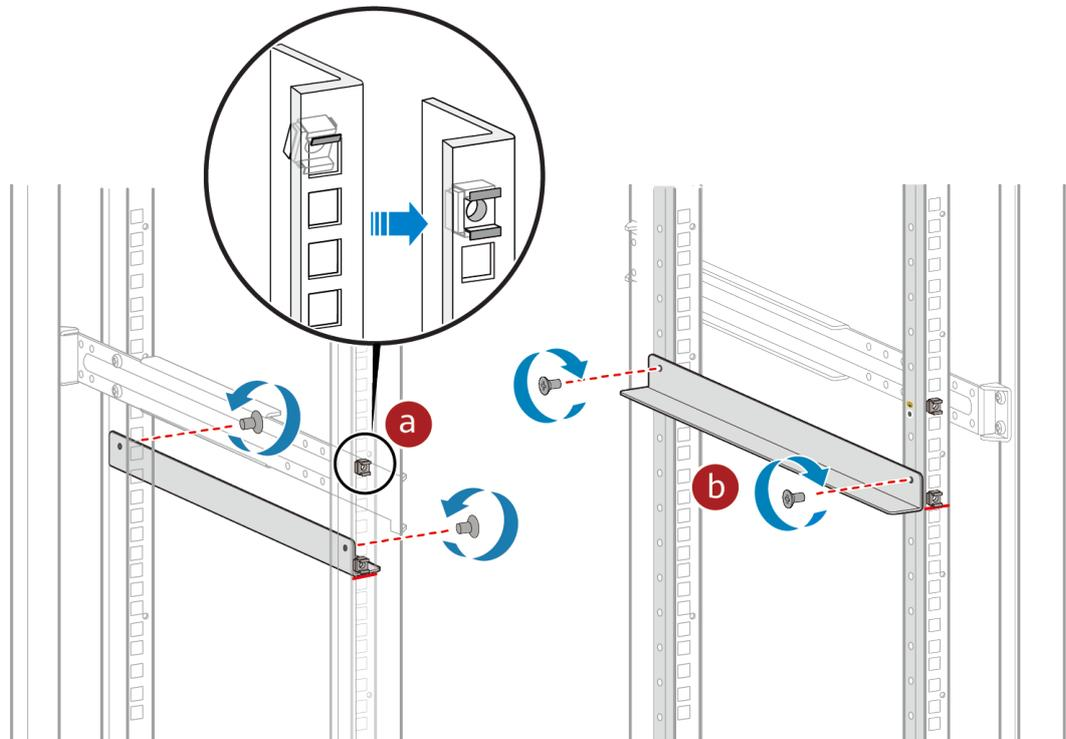
**Step 4** Install the router into the cabinet.
