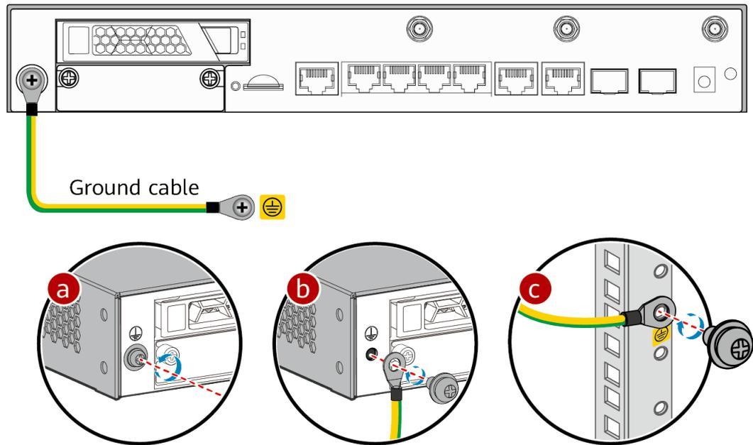
The AR651C or AR651F-Lite has the ground cable routed out from the top.
