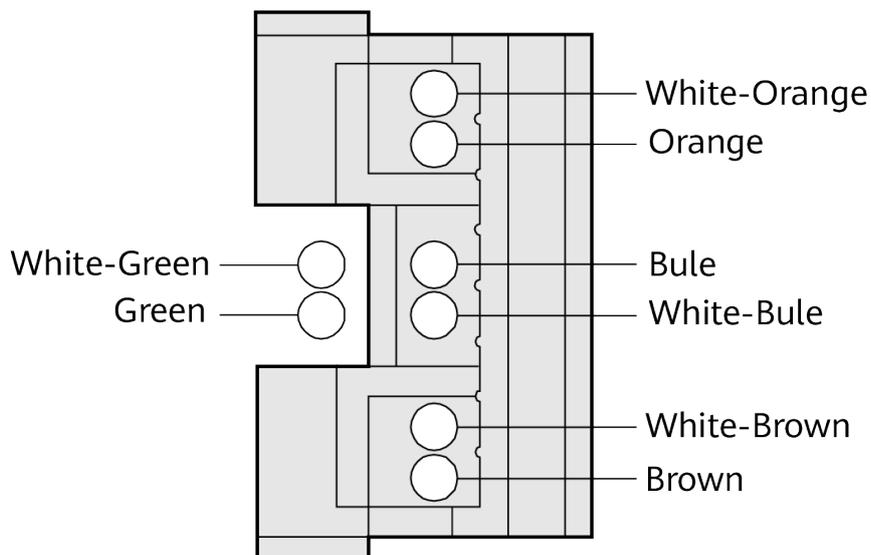
**Step 6** Align the four pairs of cables in the holder, as shown in [Figure 10-22](#). The connections between the wires and the pins are shown in [Figure 10-23](#) and listed in [Table 10-5](#).
