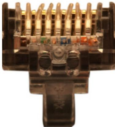
**Step 5** Hold the connector with the side facing towards you, and check whether you can see the cross-sections of the wires. Ensure that the ends of the wires are in good contact with the edge of the RJ45, and that the contact strip blade extends beyond the ends of the wires and is crimped with the wires. If not, replace the connector. [Figure 10-37](#) shows an unqualified piece.
