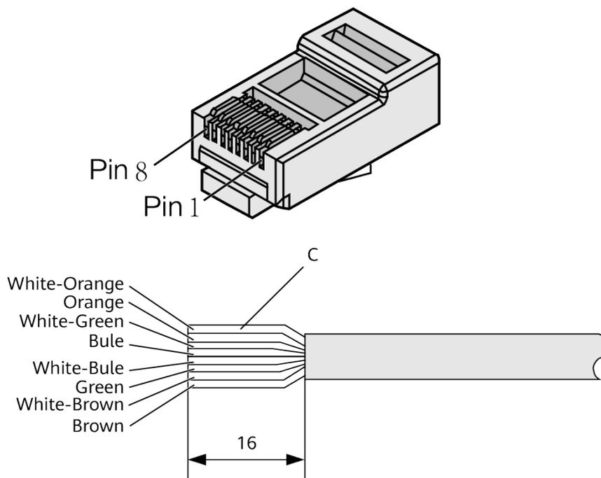
**Table 10-6** Connections between wires and pins (using a straight-through cable as an example)
