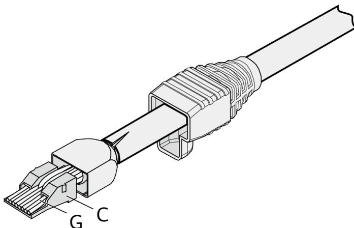
**Step 8** Put the connector body onto the wire holder and turn the metal shell by 90°, as shown in [Figure 10-25](#).
