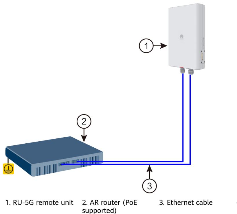
**Figure 16-4** Co-deployment Networking Mode 2 (RU-5G Powered by PoE adapters)
