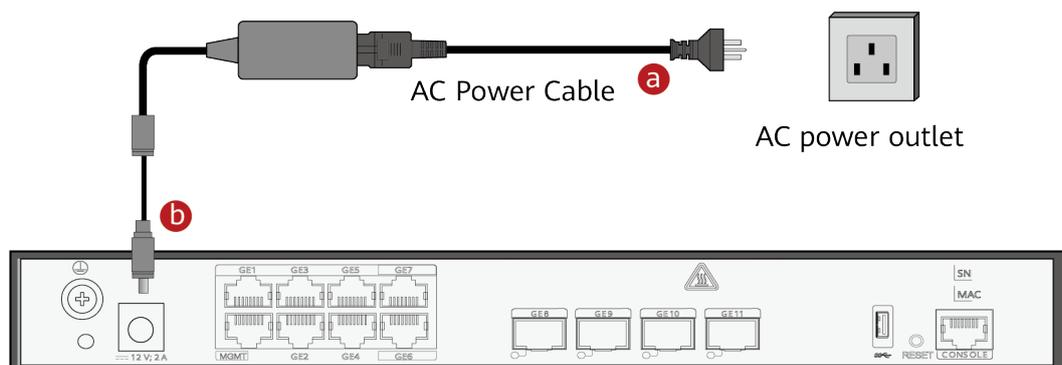
**Step 4** (Optional) Connect the AC terminal locking latch.
