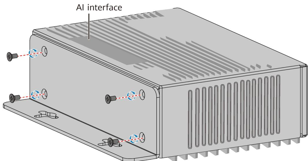
**Step 3** Mount the device on the wall.
