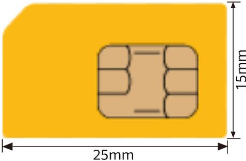
A yellow standard SIM card with a gold-colored chip. The dimensions are 25mm in width and 15mm in height.  |
