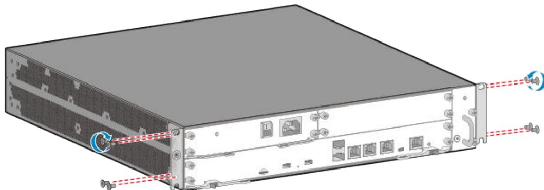
**Figure 7-2** Installing mounting brackets on an AR6300K/AR6300/AR6300-S
