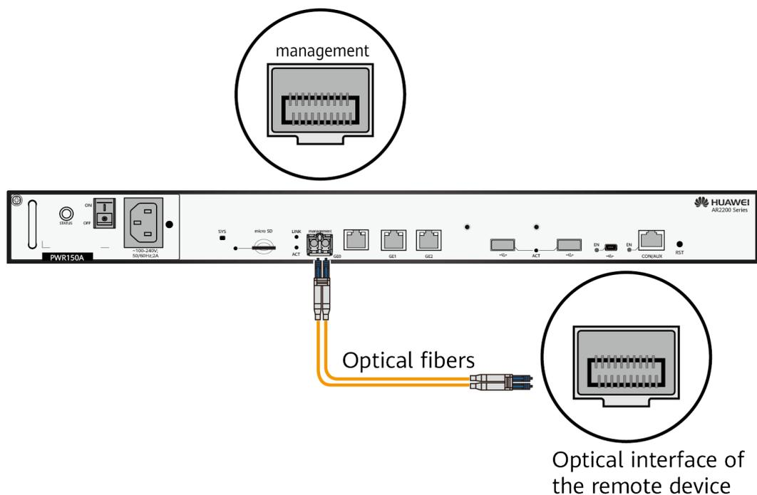
**Step 5** Arrange the optical fibers to make them parallel and bundle them with fiber binding tape at an interval of 150 mm to 300 mm.
