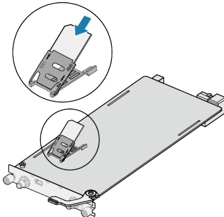
**Step 5** Slide the SIM card holder towards the direction specified by the LOCK arrow, close the SIM card holder, and tighten the screw.
