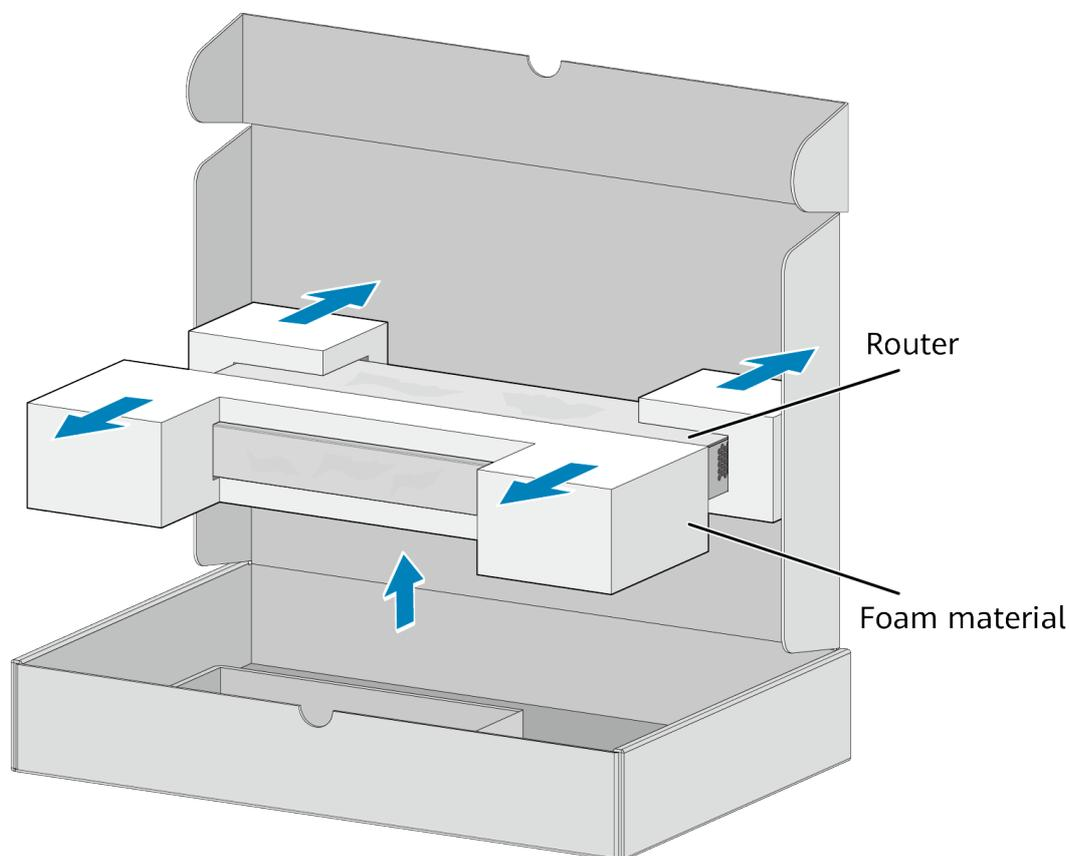
**Step 5** Take the router out of the ESD bag and check router surfaces and the warranty seal on the router. If the warranty seal is damaged, stop unpacking and contact the supplier. Huawei is unable to provide warranty services if the warranty seal is damaged or removed.
