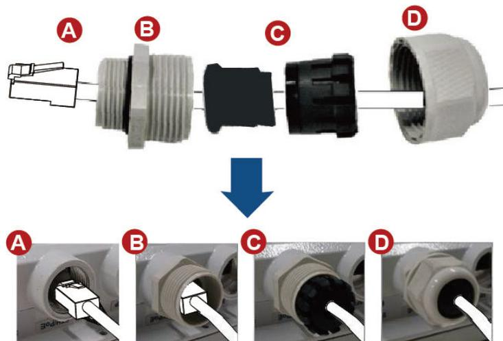
**Step 3** Connect the other end of the Ethernet cable according to the networking mode.
