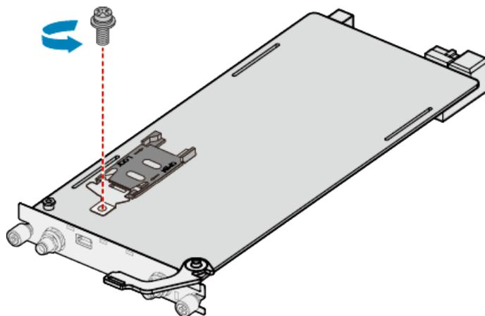
**Step 3** Slide the SIM card holder horizontally towards the direction specified by the OPEN arrow and open the SIM card holder.
