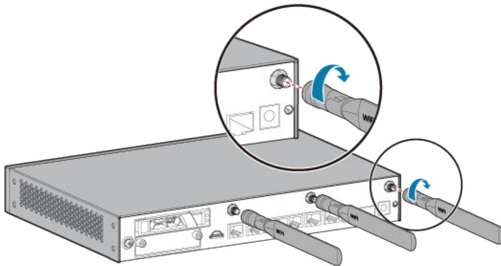
**Step 2** Make the Wi-Fi antennas vertical to the ground so that the router can better transmit and receive wireless signals.
