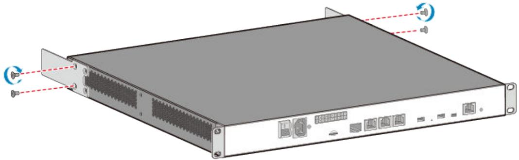
**Step 2** Install two floating nuts on each of the front and rear mounting rails. Leave a mounting hole between the two floating nuts on the same mounting rail.
