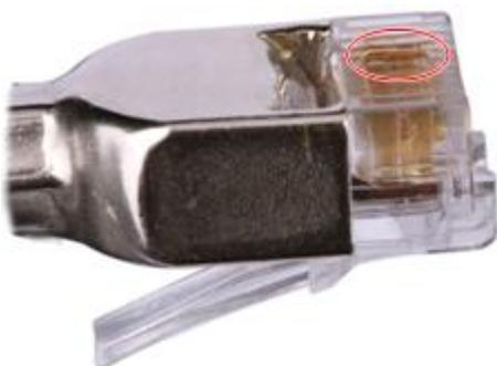
**Step 3** Check whether the contact strips are clean. If they are not clean and the dirt cannot be removed, replace it with a new RJ45 connector. **Figure 10-35** shows an unqualified piece.
