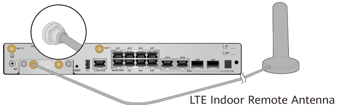
**Step 2** Fix the LTE indoor remote antennas on a metal surface that can be magnetized or keep the antennas away from the Wi-Fi antenna.
