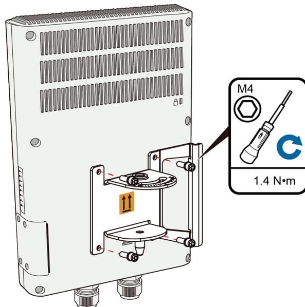
**Step 5** Remove the topmost screw from the wall mounting bracket, hang the device mounting bracket onto the topmost screw, and tighten the screw until the screw passes through the hole of the horizontal scale plate (the screw should not be too tight).
