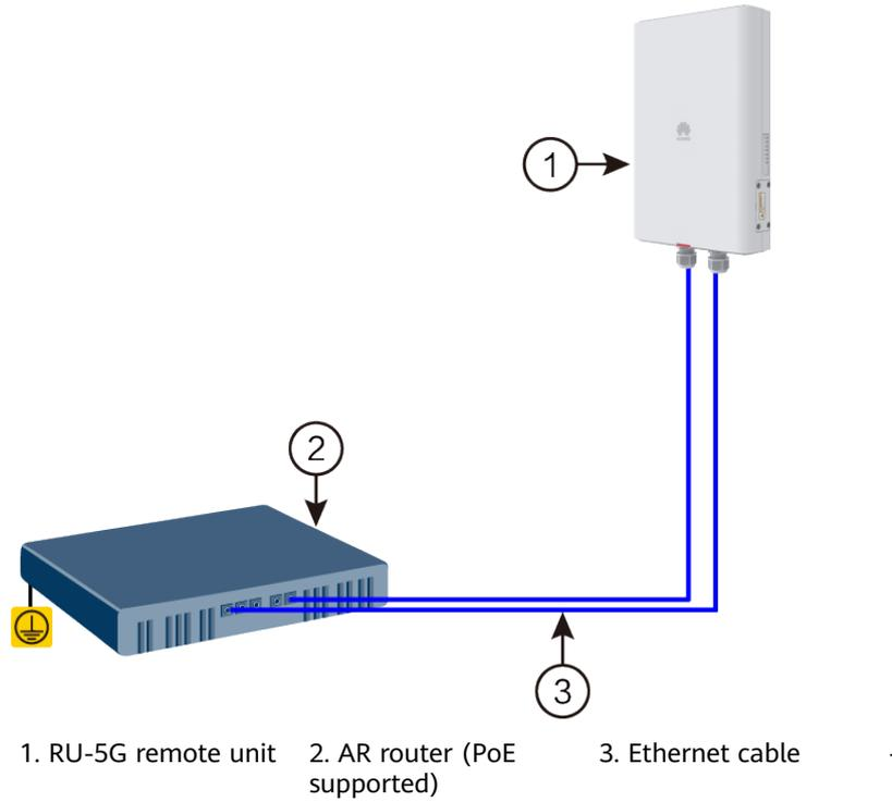
**Figure 6-4** Co-deployment Networking Mode 2 (RU-5G Powered by PoE adapters)
