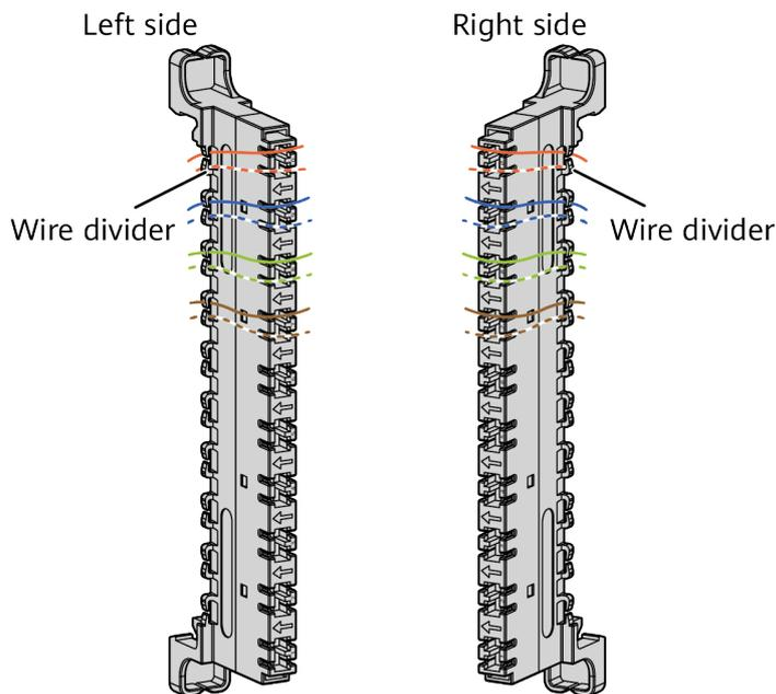
4. Use an impact tool to push the wires into the wire slots. Press a wire with the impact tool until you hear a click, as shown in [Figure 6-9](#).
