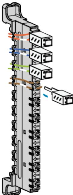
6. Install the cable management strip onto the cable management strip holder, making the end with a shorter hook face up and the end with longer hook face down, as shown in [Figure 7-12](#). Gently shake the cable management strip. If the cable management strip is still fixed on the holder, it is installed properly.
