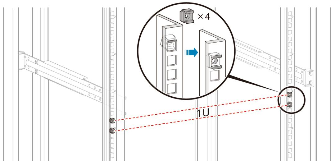
**Step 3** Move the router into the cabinet. Support the bottom of the router and tighten the M6 screws on the mounting brackets. Tighten the lower M6 screws first, and then the upper M6 screws.
