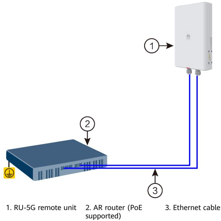
**Figure 7-6** Co-deployment Networking Mode 2 (RU-5G Powered by PoE adapters)
