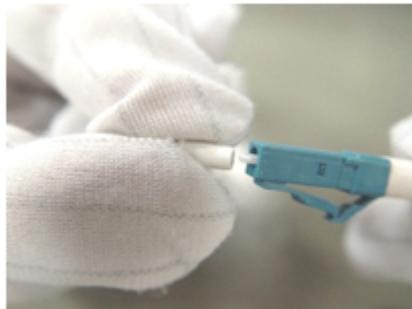
4. If a receptacle or an optical connector has not been used for a long time and is not covered with a protective cap, you need to clean it before using it. Clean a receptacle with a cotton swab, as shown in [Figure 14-6](#). Clean an optical connector with cleaning tissues.
