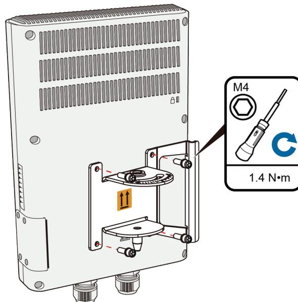
**Step 3** Remove the topmost screw from the wall mounting bracket, hang the device mounting bracket onto the topmost screw, and tighten the screw until the screw passes through the hole of the horizontal scale plate (the screw should not be too tight).
