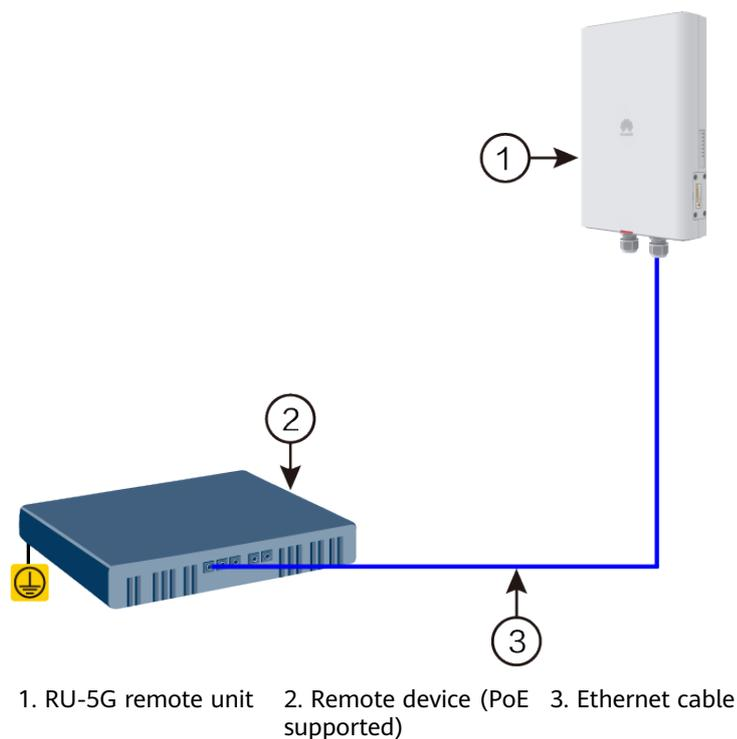
**Figure 16-6** Independent deployment Networking Mode 2 (RU-5G Powered by PoE adapters)
