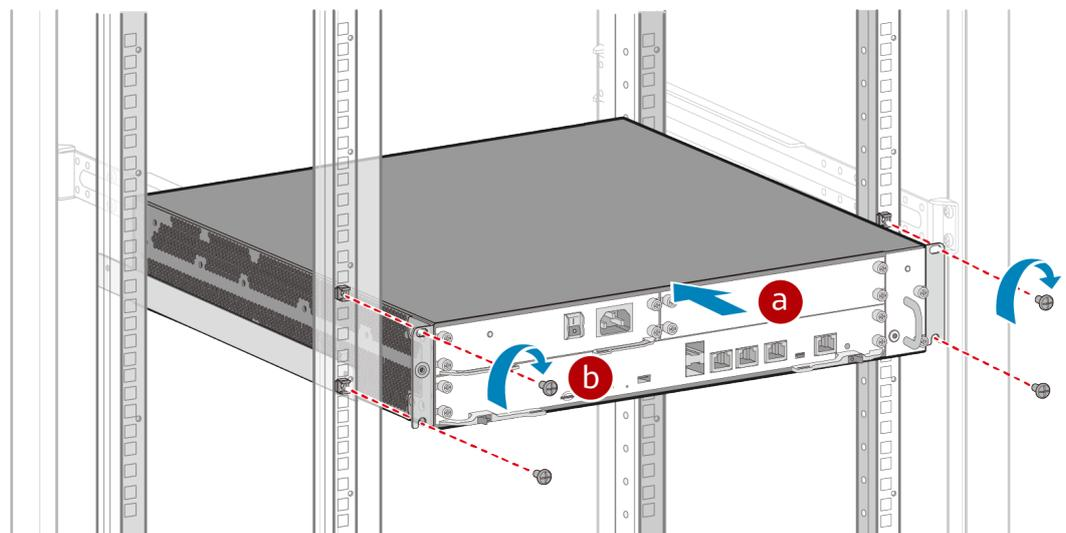
**Figure 7-4** Installing an AR6300K/AR6300/AR6300-S into a cabinet
