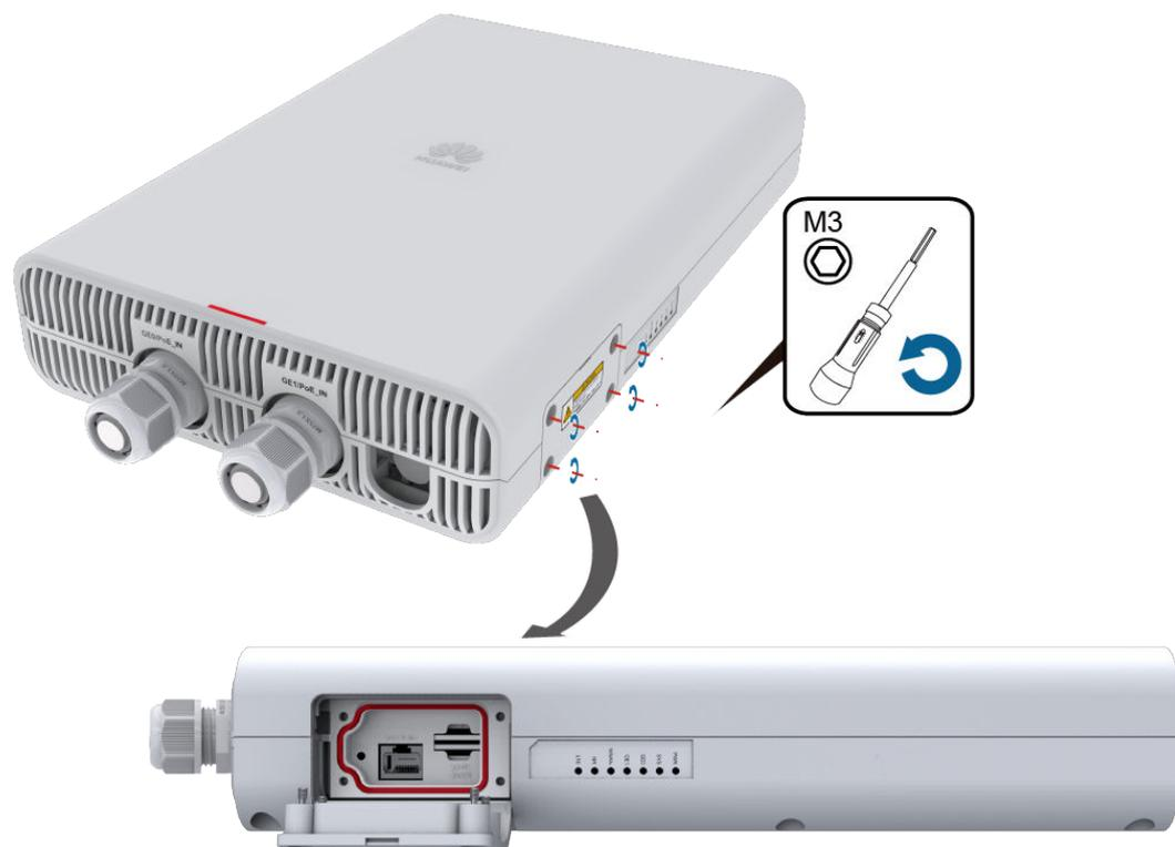
**Step 2** Place the SIM card into the SIM card slot in the direction marked on the card slot. If you hear a click, the SIM card is properly installed.
