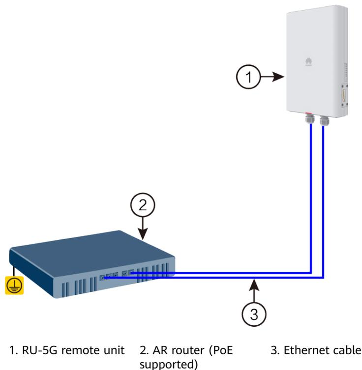
**Figure 5-2 Co-deployment Networking Mode 2 (RU-5G Powered by PoE adapters)**
