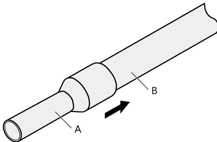
**Step 3** Crimp the joint parts of the cord end terminal and the conductor, as shown in [Figure 10-14](#).
