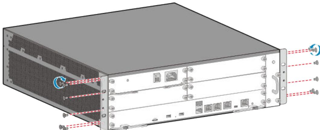
**Step 2** Mark the positions of L-shaped guide rails and floating nuts.
