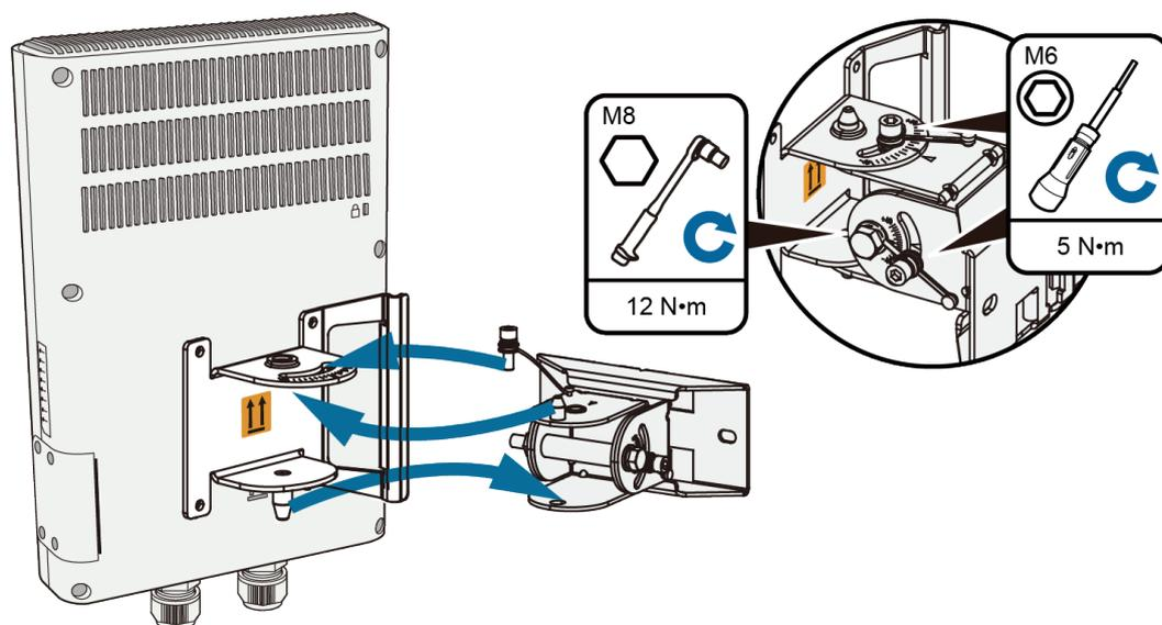
**Step 6** Loosen the two screws in the horizontal direction, adjust the horizontal and vertical angles of the device using the scale plate, and tighten all screws.
