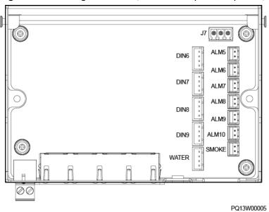
Figure 3-14 DIN and WATER pin definitions
