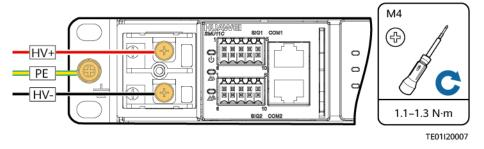
**Step 3** Reinstall the protective cover for the DC input terminals.
