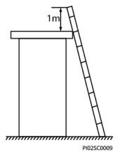
• Ensure that your body's center of gravity does not shift outside the legs of the ladder.
