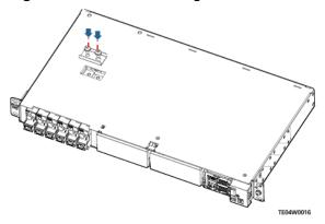
**Step 3** (Optional) Relocate the mounting ears based on the cabinet depth.
