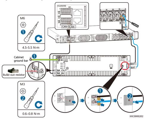
Figure 4-25 Installing lithium battery cables
