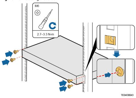
Figure 4-6 Installing a subrack
