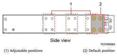
Step 4 (Optional) When installing on an ETSI rack, ensure to use the ETSI mounting ears.
