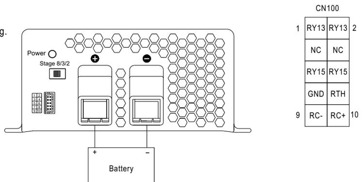
(2)Please choose the "3 stage" selection when the charger is used to charge the batteries and power the loads in the same time.
