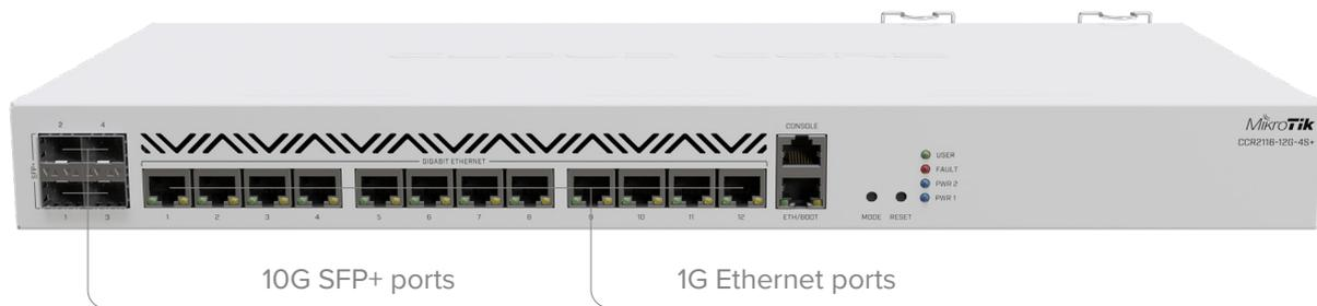
Obviously, you need the right connectivity to harness this power. There are **four 10G SFP+ ports**. They have a separate, full-duplex line connected to the Marvell Aldrin family switch chip. Then we have Gigabit Ethernet ports. 12 of them are running through the Marvel chip. And there is another Gigabit port connected directly to the CPU. For management purposes.
