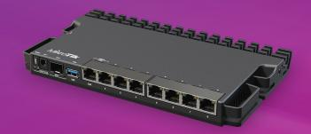
The board features 9 wired ports and a full-sized USB 3.0. Seven of the ports are Gigabit Ethernet, another one is 2.5 Gigabit Ethernet, and the last one is a 10G SFP+ cage. All the ports are connected to a powerful Marvell Amethyst family switch-chip with a 10 Gbps full-duplex line leading to the Marvell Armada Quad-core ARMv8 1.4 GHz CPU.
